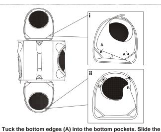
wing tips (B) into the sleeve on the top of the door.
